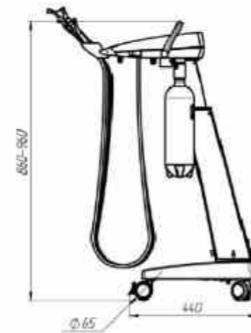
Overall dimensions of GALLANT AMBIDEXTRE dental unit: GALLANT CART-5 and 2009 NEXT patient chair.
